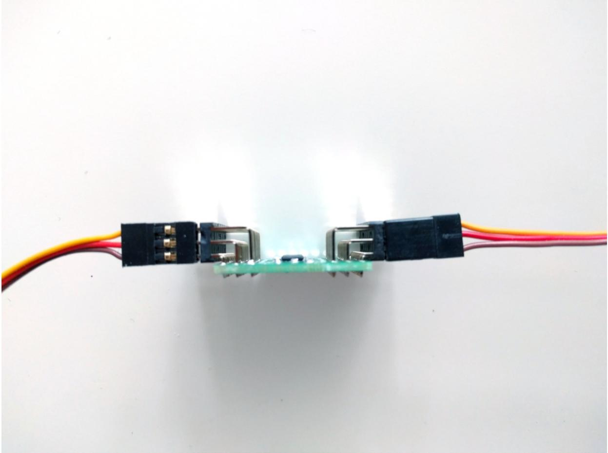
You can stack this shield with any other shields that either don't use the pins D1 and D2, or use them for I<sup>2</sup>C and have a different address than set on this shield. If you want to stack more than one servo shield on the same board, you have to change their addresses with the jumpers on the back.
