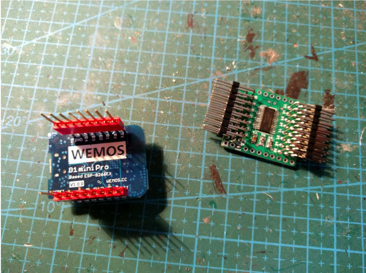
Then place the shield on the headers, making sure that every pin goes into its hole. You might need to use tweezers to help you insert all the pins.
