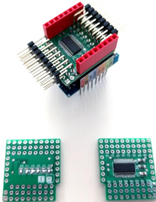
This shield is a relatively simple breakout board for the PCA9685 chip. Apart from that chip, it only contains the bare minimum of components necessary to make it work, and all the necessary connections. The goal is to make it as
