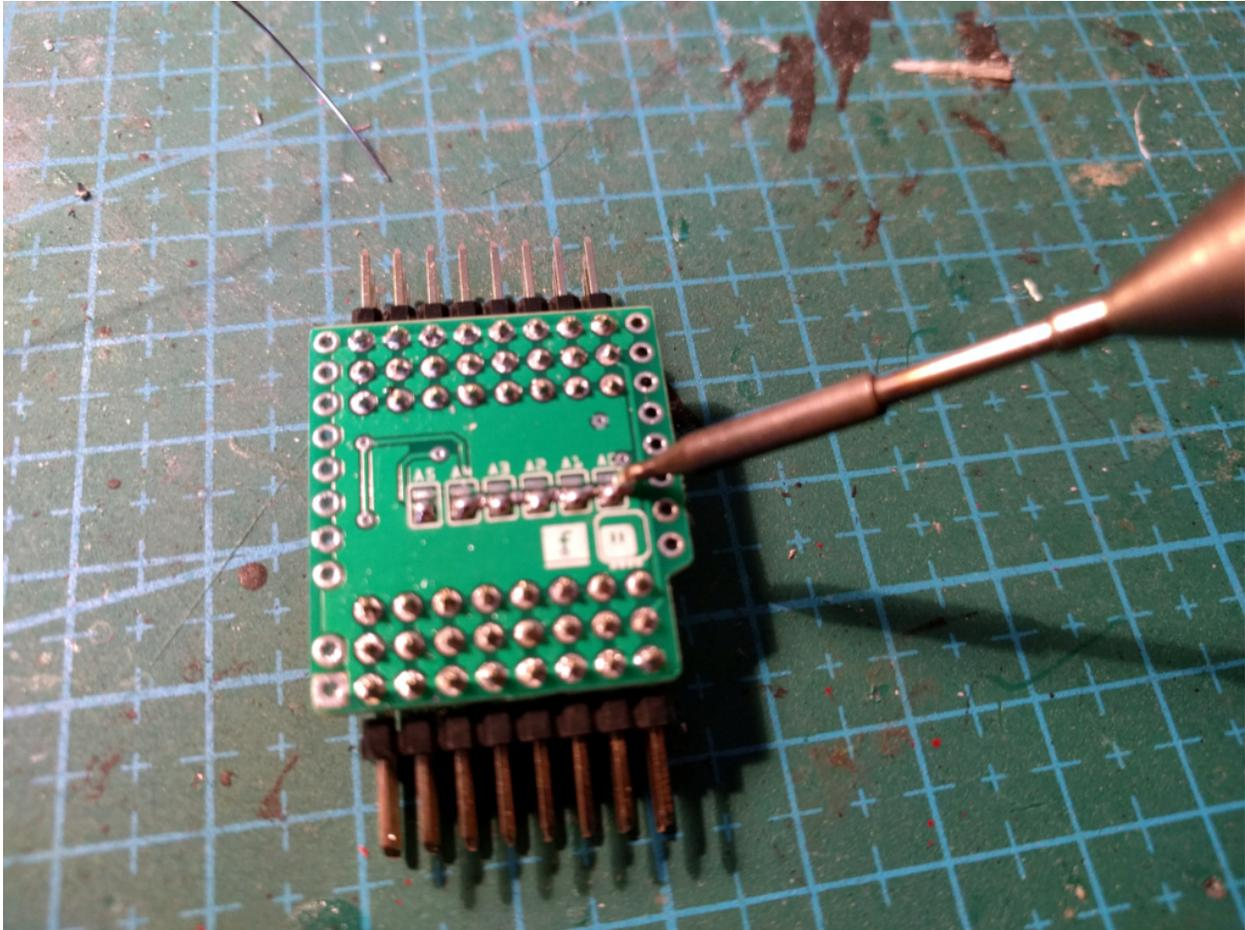
**Warning:** Be careful to not connect a jumper both to the top and bottom pads, as that will result in an electric short, a lot of smoke and possibly permanently damaged shield, microcontroller board, battery or any other power source used (including your computer, if you powered it from USB).
